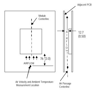
Wind Tunnel Test Setup Figure
